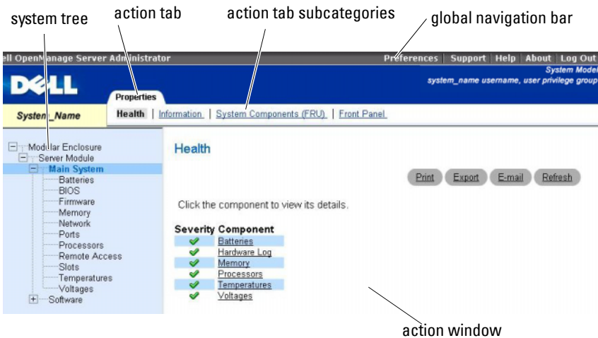
Figure 3-2. Sample Server Administrator Home Page — Modular System
